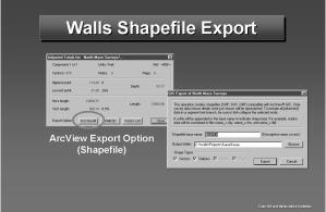
CaveTools, a free ArcView GIS extension, developed by Bernie Szukalski, converts the plot file output from Larry Fish's Compass program to shapefile format. CaveTools also allows registration of any station for which the real world coordinates are known, as well as an x, y or z shift of the shapefile.
